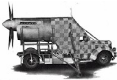
Oscar," Trans-Canada Air Lines' Merlin power-plant test truck; it is painted in vivid orange and white squares. 1952
