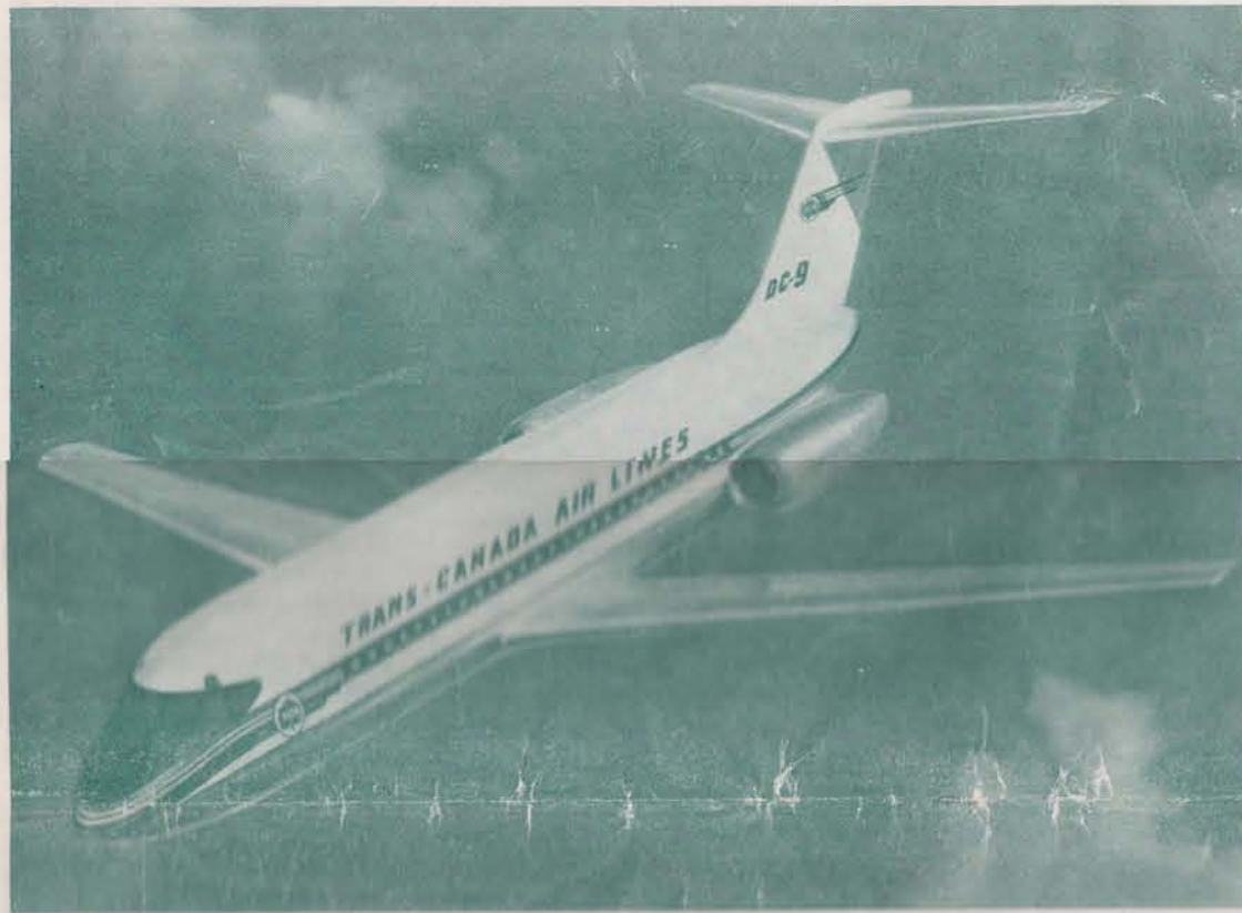
THE NEWEST BIRD in the TCA fleet of aircraft will be the Douglas DC-9. The Company has ordered six of the short and medium haul aircraft with deliveries to begin early in 1966. It will be powered by twin Pratt and Whitney JT8D-5 turbine fan engines and will cruise at 560 miles per hour at altitudes of up to 30,000 feet. It will have a cruising range of over 1,200 miles. Above is an artist's conception.
