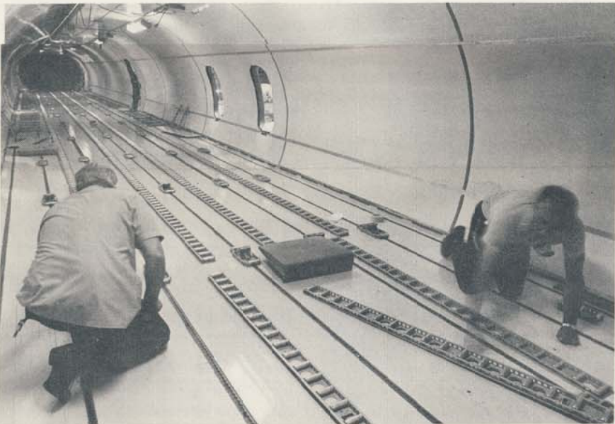
Gone are rows of faded seats. In their place are gleaming new roller beds, capable of gliding along pallets weighing up to 6033 kilos
