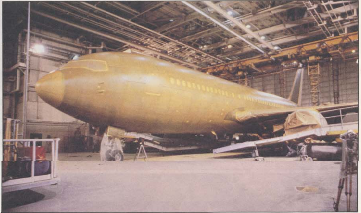
It looks like an exotic insect, but it's actually our Fin 613 sporting a coat of base paint. Once the job is complete, Boeing will have applied about 500 lbs. of paint.
