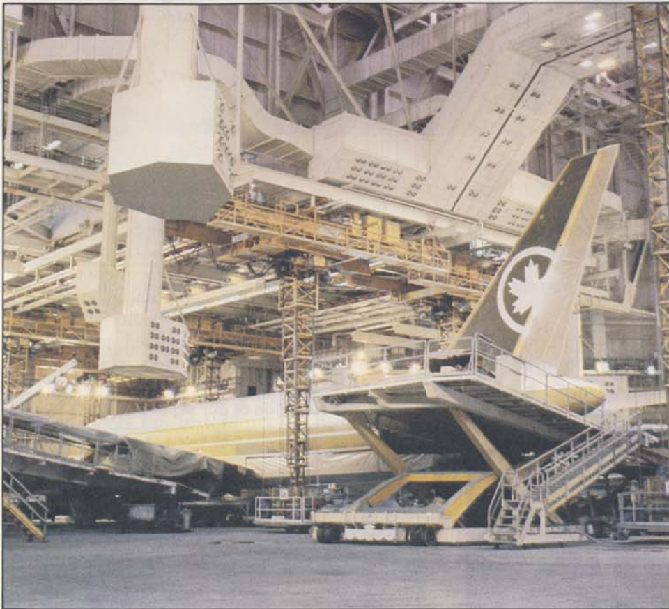
After the white and gray areas were painted, Boeing applied the red and burgundy markings.
