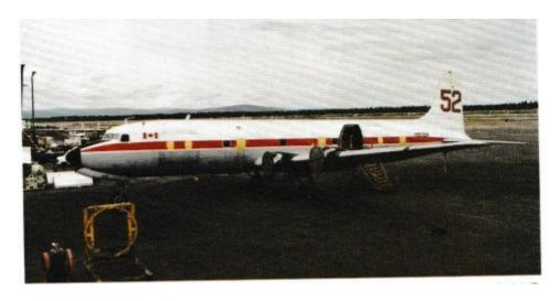
Ramp scene at Fairbanks on June 30 2001 shows Douglas DC-6A/B N9056R undergoing conversion from Conair air tanker to Everts Air Cargo freighter. All four engines had been removed and dispatched to Miami for overhaul, but once they had been installed and the aircraft given the smart Everts livery, a new chapter in her long flying career (Norbert Oertel)
